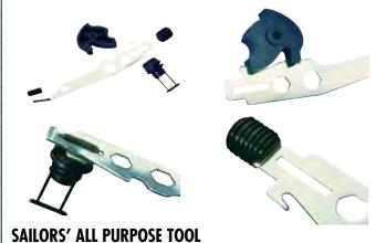
Handles screws, bolts, and shackles. Wide blade fits up into Hobie Cat's lower rudder castings for adjusting cam spring tension. Narrow blade fits the rudder stop screw and its built in hook is designed specifically to return locked "down" rudder cams to the "up" position with the twist of the wrist. 83103 EACH
