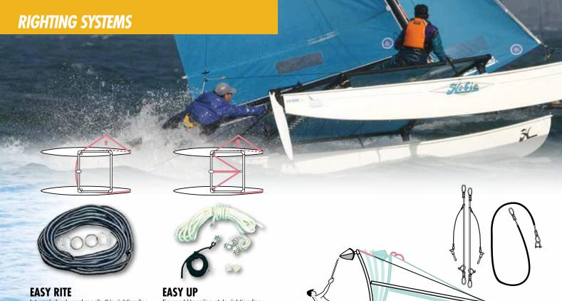
Internal shock cord recoils this righting line automatically. Made from 1/2" hollow braid line with internal shockcord. It requires no blocks or shackles. Installs in minutes without tools. Also functions as crew safety line. Our best selling righting system.
