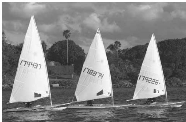
Your boat rigged will resemble one of the Lasers shown above. From left to right: Laser, Radial, and Laser 4.7.
