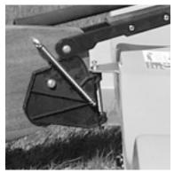
Rudder & Tiller Assembled and mounted
